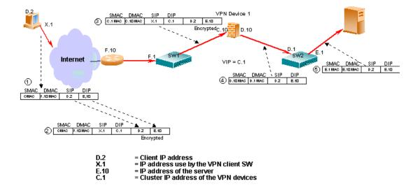
Figure 14-1 Basic Network Frame Flow and Operation
